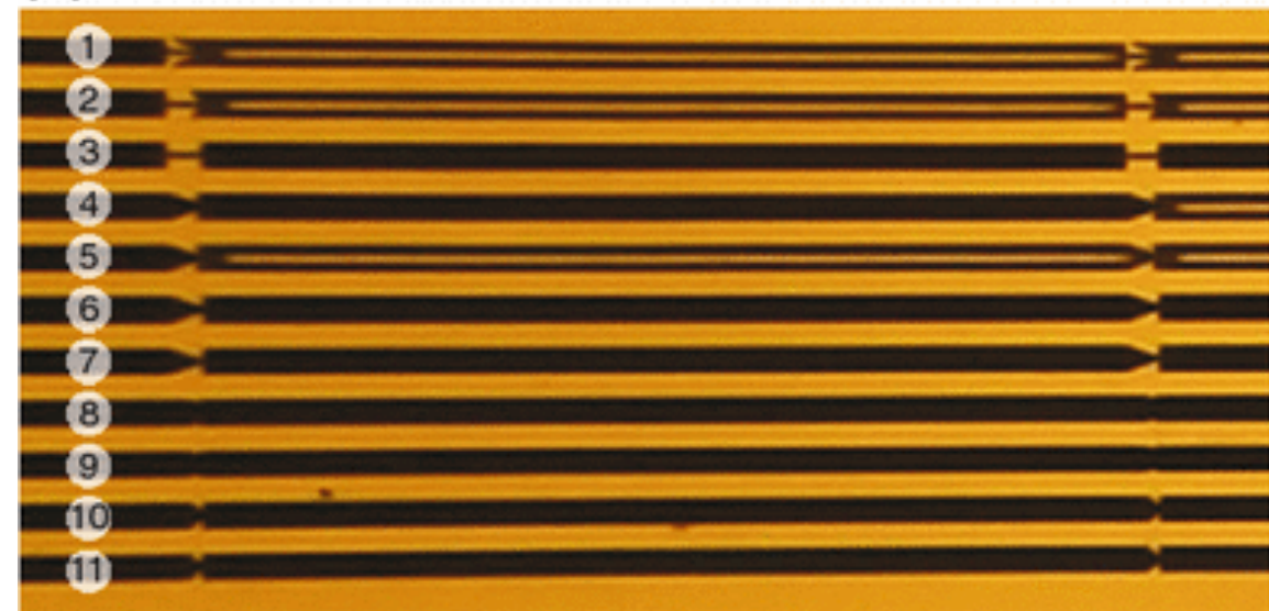
(b) Stop valves etched in silicon
